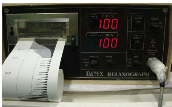
Fig. 2 – Electromyograph. Relaxograph NMT Monitor (Datex Instrumentarium Corp., Helsinki, Finland). Recording strip with real time TOF. Source: Authors.
